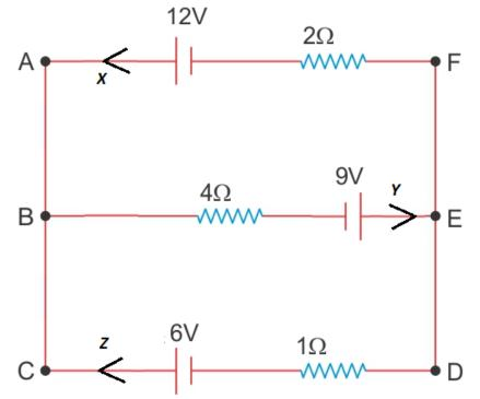
Three unknown currents: x, y, and z are identified in the above circuit. 1. Write down the junction rule equation using the assigned currents.
